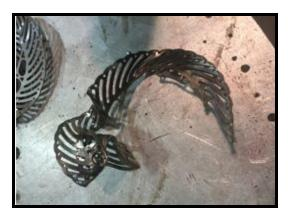
This year was the first year where we had fully customized the cutting brakes. The FOS for OD12's rear rotors were determined using hand calc (Check my tech report from Fall 2015). During competition this year one of the rotors was torn off the hub, but we
